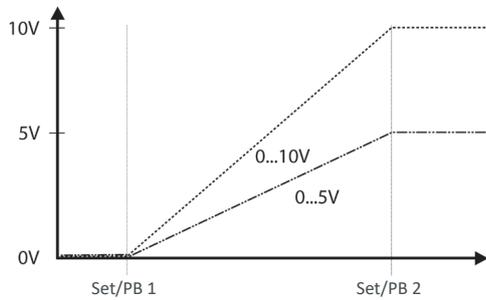
Configurable version V with Limit Switch function
