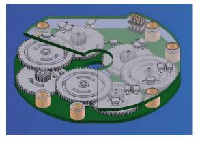
Linear systems normally need more than one turn of a shaft. A single turn encoder is unsuitable for this type of application because of the additional requirement of the number of turns. The principle is relatively simple: Several single turn encoders are connected using a reduction gear. The first stage supplies the resolution per turn, the stages behind supply the number of turns. In the following picture you can see the gearing module with the several stages of reduction gears.
