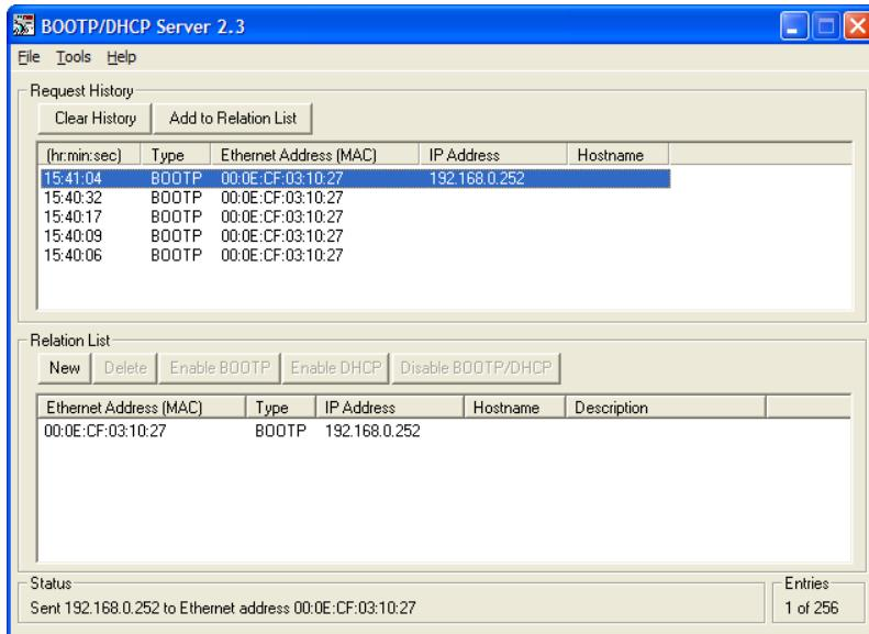
After setting the IP-Address with this tool the IP-Address will be available only after the next BOOTP request.
