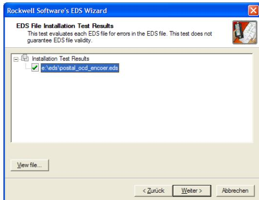
The Wizard finds all EDS files that are discarded in the choosing path and operates a test to check the EDS files on errors. In the next step pictures can be selected for the using nodes. With the button *weiter* the installation can be continued and finished.
