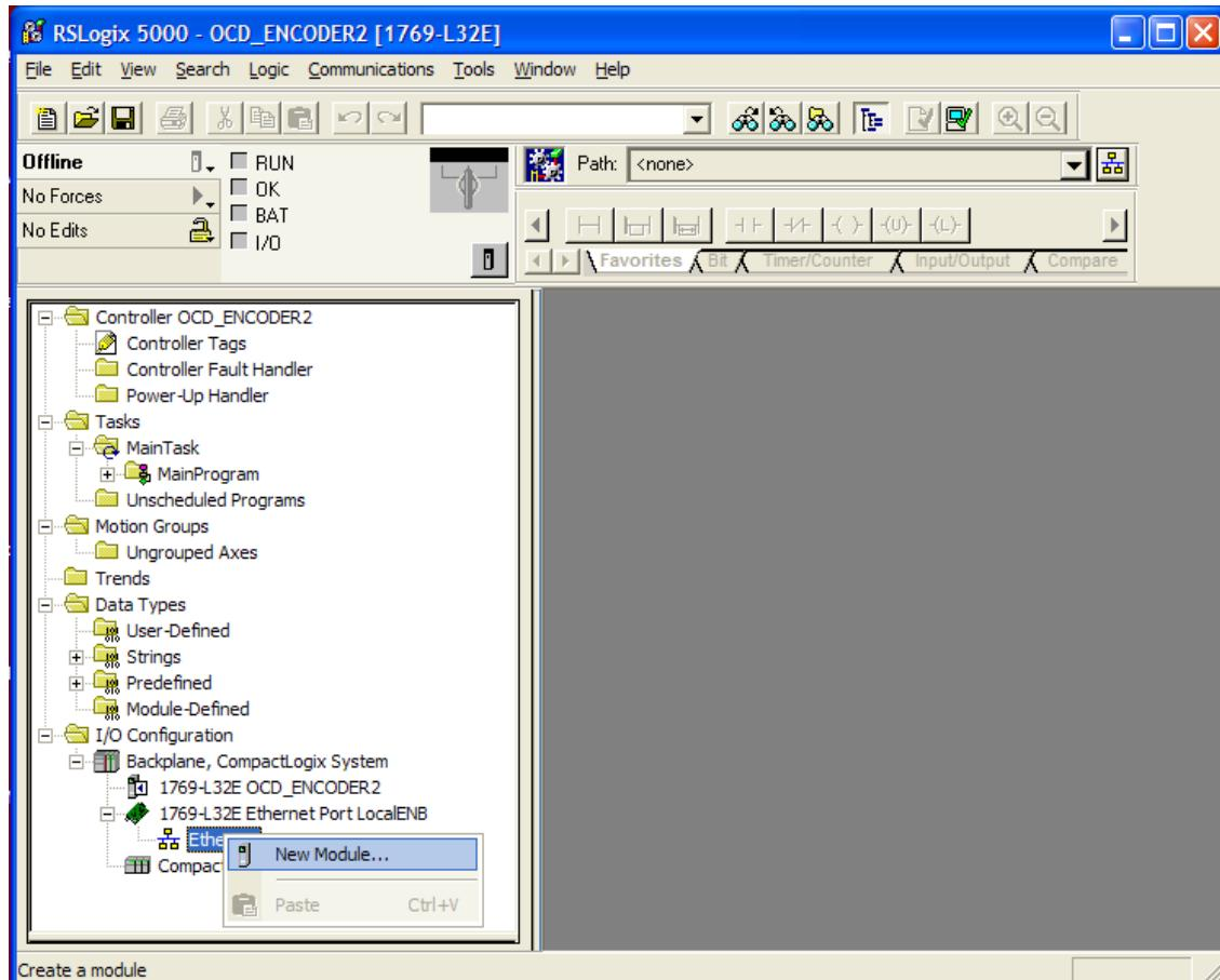
For using a Generic Device select the Generic Ethernet Module. Some PLC's support Encoder Devices too. Please check that the matching
