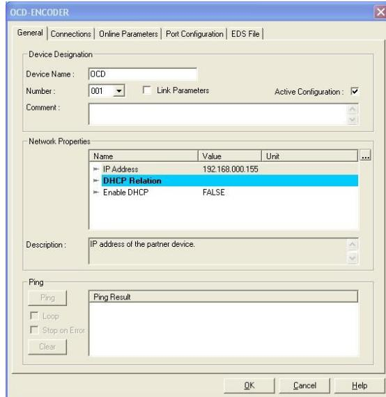
In tab *Connections* under *General* can be checked the cycle time (RPI), the input and output configuration. Under *Configuration*
