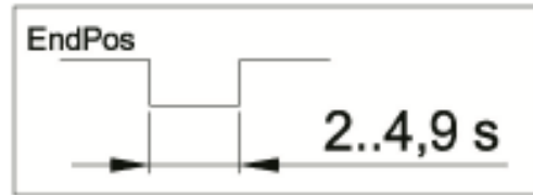
Picture 5. Setting of the end position and closing the angle adjustment mode.
